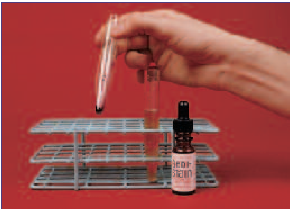
Figure 2.1 After centrifugation, the supernatant is decanted by inverting the tube. Approximately 0.5 ml of liquid is left in the tube. An equal volume of stain (0.5 ml) is added to the remaining sediment and gently mixed.
