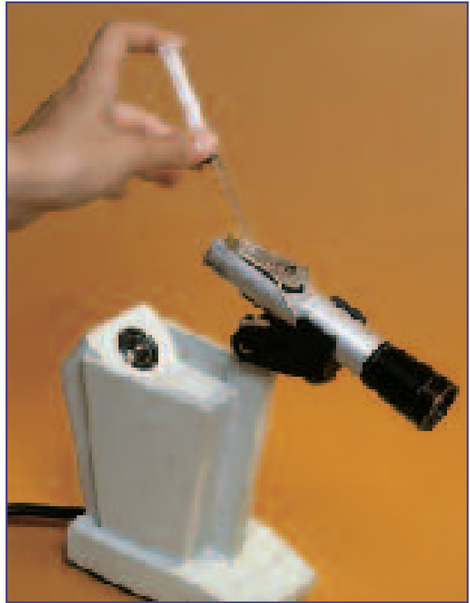
Figure 3.4 A drop of the patient's urine is placed on the refractometer to measure specific gravity.
