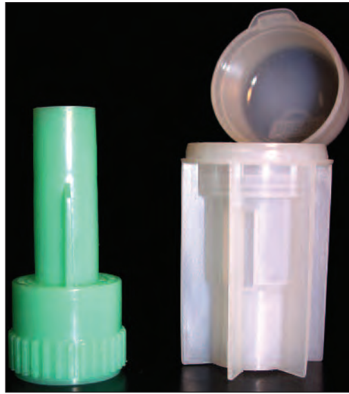
Figure 1.7. The Fecalyzer is a stationary flotation device that has been developed for the collection and processing of fecal samples. The internal portion can be used to collect a portion of feces of appropriate size by inserting the end into the feces. The sample can then be placed into the outer container and brought into the clinic. When it is time to examine the sample, flotation medium can be added and the sample mixed by twisting the insert inside the holder. The insert is then filled with flotation solution so that a positive meniscus is formed. A sieve in the insert prevents large particles from floating to the surface. A 22 × 22-mm coverslip is then placed on the top of the tube, and it is allowed to sit for 5 to 10 minutes. The coverslip is then removed and placed on a microscope slide to determine what parasites have floated to the surface.
