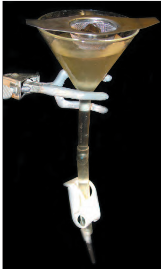
Figure 1.15. This device consists of a funnel attached to a piece of rubber tubing with a clamp. Fecal material is placed in a piece of gauze or a tea strainer and is suspended in water in the funnel. Larvae migrate out of the feces and into the water. With time, the larvae will settle to the bottom of the tube and can be harvested either by placing a drop out of the tip onto a slide or by spinning the contents down in a centrifuge tube and examining the sediment.
