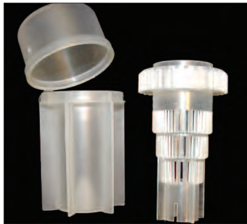
Figure 1.8. The Ovassay is a fecal collection and processing device used to perform a stationary fecal flotation. The internal device can be used to collect a sample of appropriate size by stabbing it into the feces. The insert can then be placed into the holder and brought to the clinic. When it is time to process the sample, flotation medium can be added to the tube, and the feces is mixed with the medium by twirling the insert in the holder. The insert is then filled with flotation medium until a positive meniscus is formed. A 22 × 22-mm coverslip is then placed on the meniscus, and the device is allowed to stand for 5 to 10 minutes. The coverslip is then removed and transferred to a microscope slide to identify those parasite stages that have floated to the surface.
