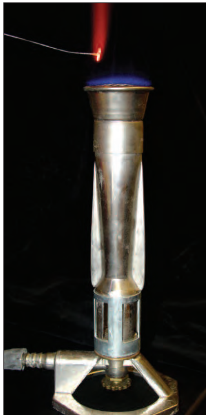
Figure 1.6. The loop used to pick up a specimen from the top of a tube is finer than the typical microbiology loop with a somewhat larger diameter. It is important that the loop be made from wire that is resistant to flame, or it will melt when it is flamed. The flaming seems to help the loop collect the sample from the meniscus of the centrifuged tube. Occasionally the loop will accumulate a crust of dried material from the feces and flaming that can be carefully broken off the wire using the end of an applicator stick.
