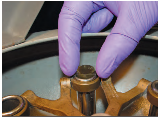
Figure 1.12. After the centrifuge comes to a complete stop, the coverslip can be lifted directly from the top of the tube.
