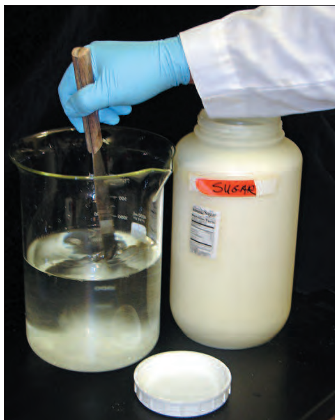
Figure 1.9. When preparing sugar for flotation, typically about 900 g (2 lbs) is needed for every 700 mL of water (need about 1300 g/L). It will be necessary to slowly add the sugar to the water and dissolve it by stirring. Often the water can be warmed to help in the dissolution of the sugar, but it should be cooled before the specific gravity is checked with a hydrometer. Some find it very useful to prepare the sugar solution in a double boiler just like when making candy. It is a good idea when the product has cooled to add a small quantity of formalin (10 mL/L) to prevent mold from growing in the medium.
